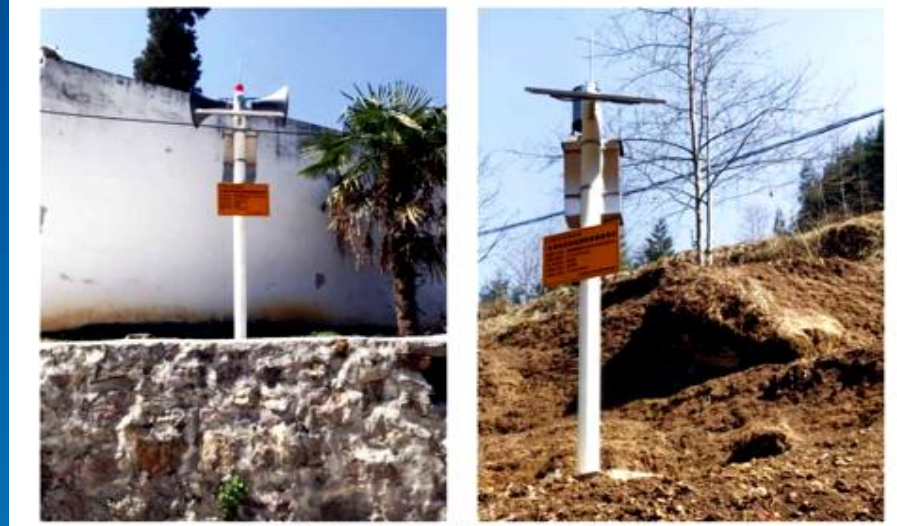
凉山州甘洛县海棠城海棠村4组大树湾泥石流雨量监测及无线预警广播
