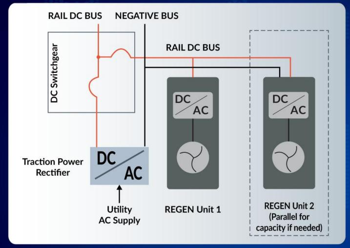
VYCON's REGEN Energy Recycling flywheel system uses a permanent magnet motor generator design and levitates within an electromagnetic field a perfect environment for producing short duration, highpower discharges. It's the reason VYCON's flywheel energy storage systems can charge and discharge at high rates for countless cycles, and why it's making conventional technologies obsolete.
